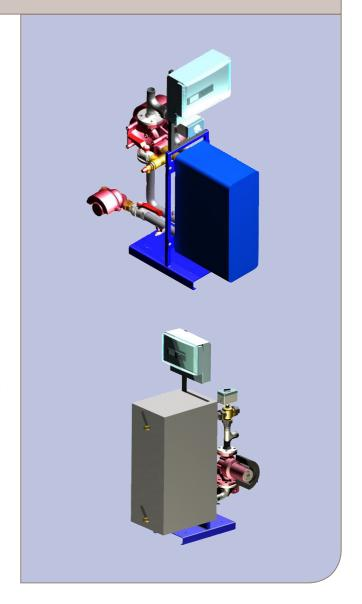
A circulation pump - which is usually used to limit the time needed to deliver domestic hot water to the tap at the right temperature- maintains a constant flow rate through the heat exchanger and through the distribution pipe-work.
